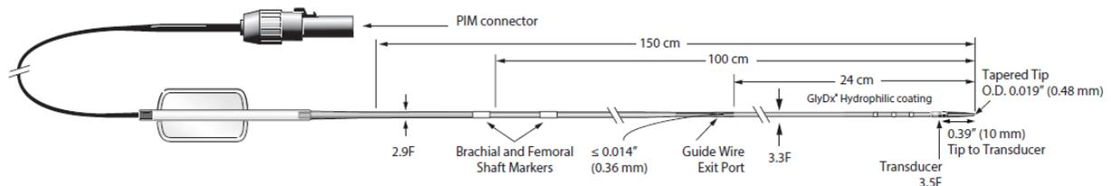
Figure 1: Eagle Eye Platinum RX Digital IVUS Catheter
